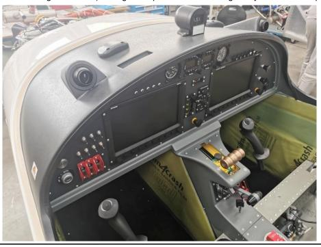
**4.** Loosen the 4 screws in the corners of the SkyView display with a size 2 hex screwdriver. When unscrewing the 2 middle screws, hold the SkyView display to prevent its falling and damage!
