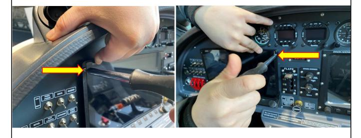
2. Once the display is screwed in, take a drill with a Ø 3.2 mm drill bit and mark the bottom holes for mounting the display by short drilling into the dashboard.
