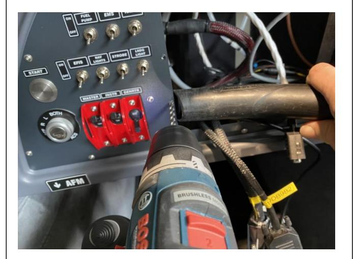
**5.** After drilling the holes, the mounting of the rivet nuts follows. Special pressing pliers are then used to carefully press the nuts onto the dashboard. Use the M3x10 riveting nut series 39006 and respective extender for riveting pliers. When pressing, take care to exert sufficient force on the pliers to press the nut firmly enough, but at the same time not to destroy it by stripping the threads.
