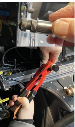
**6.** After pressing the nuts, mount the "filler" Panel Plate (P/N 102897-000) /1/ by attaching it with the two socket screws (use the screws M3x12 AN9084 A2 with the original display installation) by a size 2 hex screwdriver.
