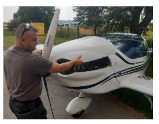
Release the upper cowling from the crews and pull it forward (in the flight direction). Then lift it evenly on both sides.
