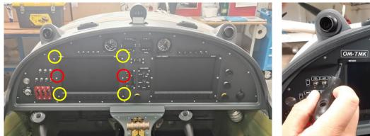
Take the SkyView display out of the instrument panel. On its rear side, after releasing the plastic lock, disconnect the Ethernet connector, then the USB connector, and all 3 data D-sub connectors (SVL10DB9B-1, SVL10DB9B-2, SVL10DB37B), secured by screws on the connectors' bodies. Place the SkyView classic SV-D1000 display on the shelf.
