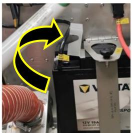
Disconnect battery terminals from onboard electric bus before you start working with the electric system! Loosen and unscrew the hex screw with a nut on the minus pole of the battery – the black cable on the right side of the battery (in the flight direction). Use a 10 mm open-ended/ring spanner for the loosening. Place the loosened black cable away from the battery's minus pole, so that its accidental release and a restored contact with the minus pole of the battery is prevented.
