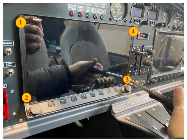
9. Repeat the entire installation procedure for the second display. After mounting, it is necessary to upload the data from the backup to the individual displays. Upload the backup from the right SkyView D1000 to the right SkyView HDX 1100. And upload the backup from the left SkyView D1000 to the left SkyView HDX 1100. Instructions for restoring the backup must be done from the installation manual for the SkyView HDX 1100 /1/.
