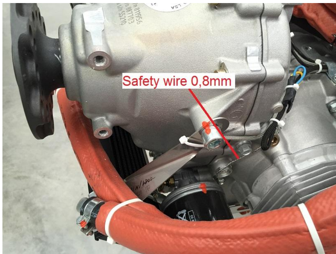
Figure 9: Stainless safety wire application
