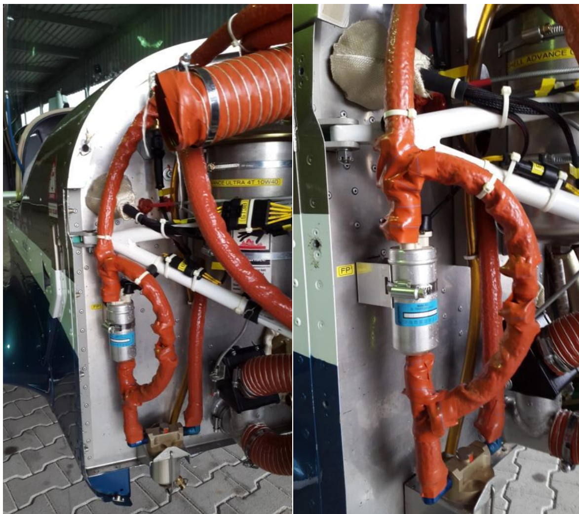
Figure 24: Left (firewall right side overall look) Right (electric fuel pump closer look)
