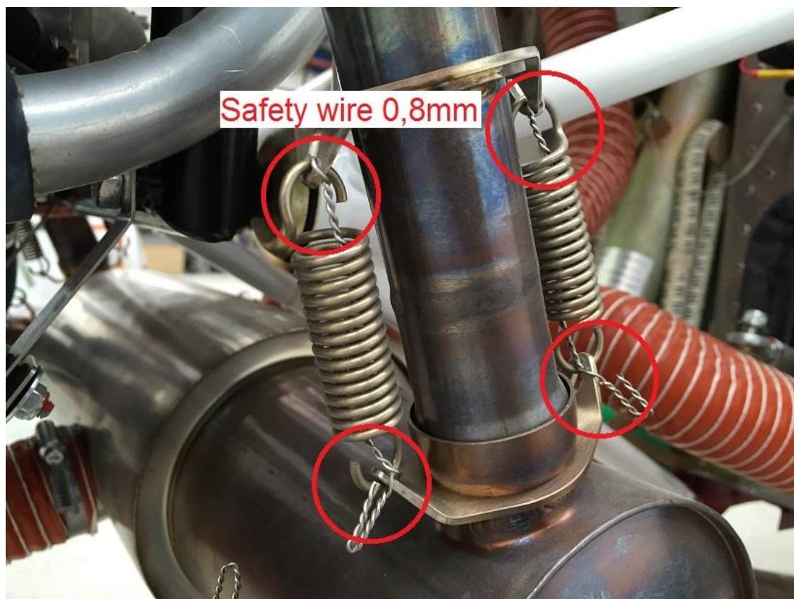
Figure 10: Exhaust tubes connection secured by 0,8mm stainless wire
