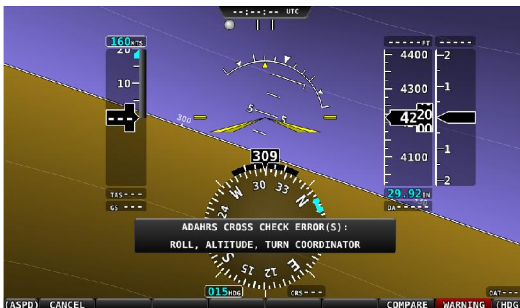
Figure 54 - ADAHRS Cross-Checking Disagreement
